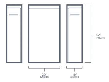
The NeoVolta NV24 is an additional 9,600 W battery capacity option that combines with the NV14. Total energy storage capacity is increased from 14.4 kWh to 24.0 kWh of Lithium Iron Phosphate (LiFePO4) rechargeable battery. The NV24 weighs 280 pounds and has to be ground mounted.
